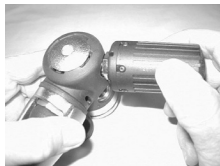
Fig. 132 -INSTALLING A TRT ON A REGULATOR
