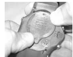
Fig. 109 - ALT BATTERY HATCH INSTALLATION
