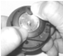
Fig. 106 -ENGAGING the RETAINING RING TABS
