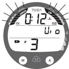
Fig. 66 - VGM MAIN (on surface)
