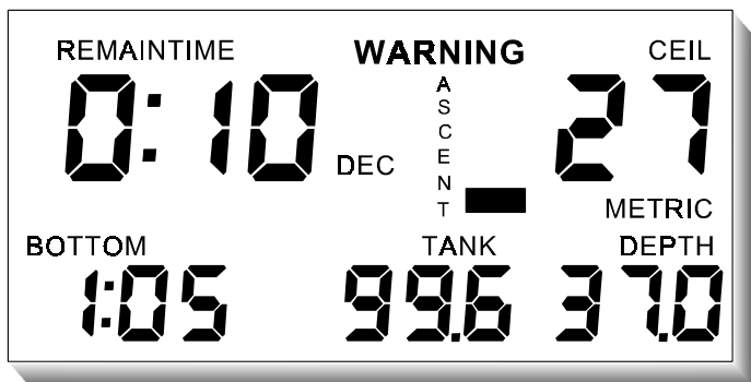
Fig-10a Primary Display, Showing a 27-meter Ceiling
