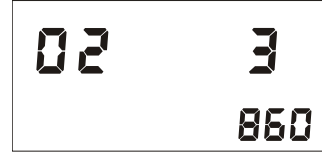
Figure 281aH PROGRAMMING MODE (Constant FO2 Mode) (Helium Enabled) (Setting Blend #3 Oxygen %)
