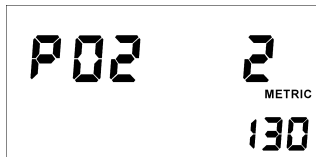
Figure 32 PROGRAMMING MODE (Constant PO2 Mode) (Setting Deco PO2 Value) Set Point PO2 1.30 ata
