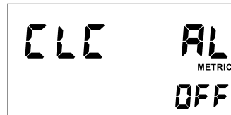
Figure 41a PROGRAMMING MODE (Clock Alarm - On/OFF)
