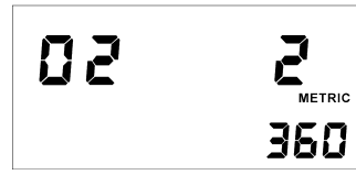
Figure 28H PROGRAMMING MODE (Constant FO2 Mode) (Helium Enabled) (Setting Deco Blend Oxygen %) Oxygen Percentage 36 %
