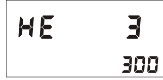
Figure 321H PROGRAMMING MODE (Constant PO2 Mode) (Helium Enabled) (Setting Blend #3 Value) Set Value 30 %
