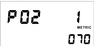
Figure 31 PROGRAMMING MODE (Constant PO2 Mode) (Setting PO2 Value) Set Point PO2 070 ata
