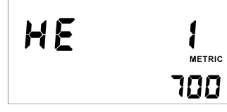
Figure 31H PROGRAMMING MODE (Constant PO2 Mode) (Helium Enabled) (Setting Blend #1 Value) Set Value 70 %
