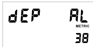
Figure 25 m PROGRAMMING MODE (Setting Depth Alarm) Depth Alarm 38 meters
