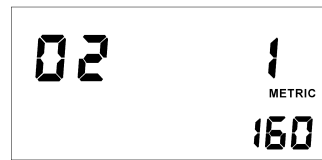
Figure 27H PROGRAMMING MODE (Constant FO2 Mode) (Helium Enabled) (Setting Blend 1 Oxygen %) Oxygen Percentage 16 %
