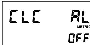
Figure 41a PROGRAMMING MODE (Clock Alarm - On/OFF)
