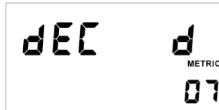
Figure 30 PROGRAMMING MODE (Constant FO2 Mode) (Setting Deco Blend - Depth Benchmark) Depth 7 mtr
