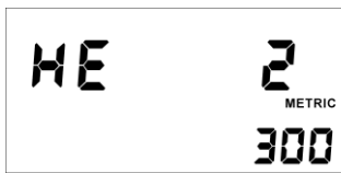
Figure 32H PROGRAMMING MODE (Constant PO2 Mode) (Helium Enabled) (Setting Deco Value) Set Value 30 %
