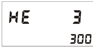
Figure 321H PROGRAMMING MODE (Constant PO2 Mode) (Helium Enabled) (Setting Blend #3 Value) Set Value 30 %
