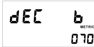
Figure 29 PROGRAMMING MODE (Constant FO2 Mode) (Setting Deco Blend - Time Benchmark) Bottom Time 70 min.
