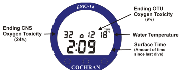
Figure 29a LOGBOOK MODE DECOMPRESSION (Alternate Screen)
