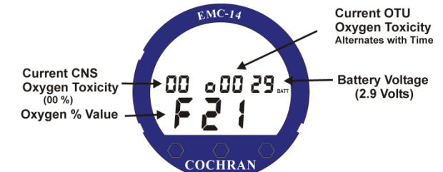
Figure 03a SURFACE MODE ALTERNATE SCREEN Without Nitrogen Showing OTU
