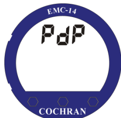
Figure 12 PROGRAMMING MODE (PreDive Prediction Menu)
