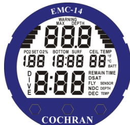
Figure 01 DIAGNOSTICS DISPLAY (Unit Turning On) All Segments Illuminated
