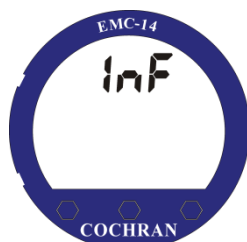
Figure 14 PROGRAMMING MODE (Information Display Menu)
