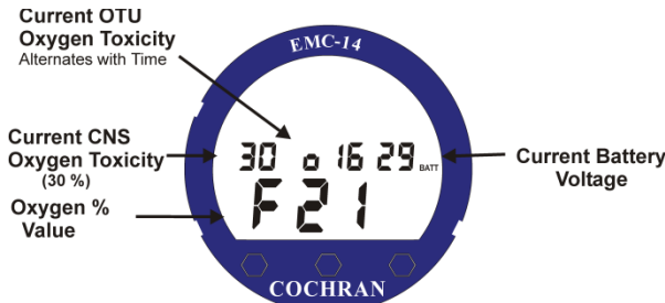
Figure 05 SURFACE MODE ALTERNATE SCREEN With Nitrogen Showing OTU
