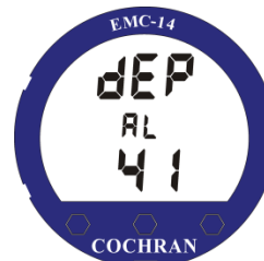
Figure 16 PROGRAMMING MODE (Depth Alarm Menu)
