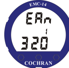
Figure 20 PROGRAMMING MODE (Setting Oxygen % Menu)
