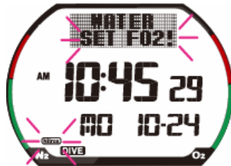
Default warning indicated by ‘Nitrox’ and upper display blinking, with an audible alarm
