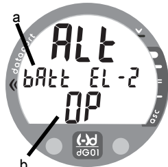
Fig. 5 - BATTERY STATUS (OP = Operable)
