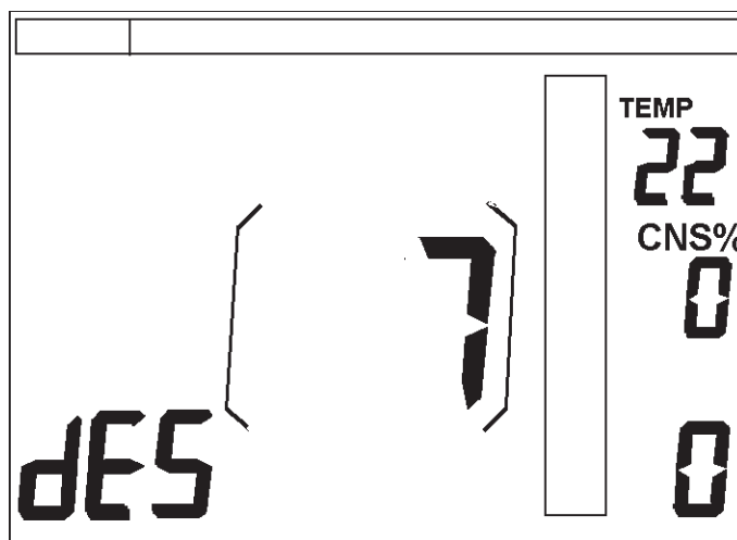
Figure 9: Desaturation Time Display The third and last surface display of the NiTek 1 is the desaturation time display, that gives the diver the time to desaturate, in hours and minutes. The NiTek 1 desaturation time is calculated to normal sea level pressure plus pressure equal to one half foot of sea water. The desaturation time can also be considered as do-not fly time.
