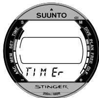
Fig. 2.6. The Stopwatch function is indicated by the TIMER text and a mode indicator.
