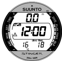
Fig. 3.25. Surface display. Alternating display showing the no-flying time.
