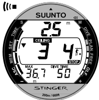
Fig. 3.14. Violated Mandatory Safety Stop. Downward pointing arrow and an audible alarm indicate you should descend to ceiling zone.
