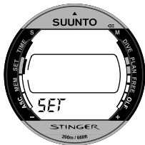
Fig. 4.1. The Setting Mode is indicated by the SET text and mode indicator.
