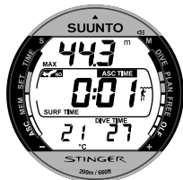
Fig. 3.26. Surface Mode after a violated decompression dive. ASC TIME symbol indicates that you have violated the ceiling for more than three minutes. The alternating display shows you that you must not dive again for at least 48 hours.
