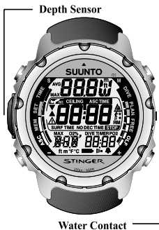
Fig. 2.2. The water contact and depth sensor.
