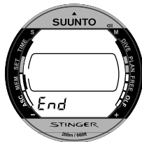
Fig. 5.7. Logbook, end of the memory. END text is displayed after oldest and the most recent dive.
