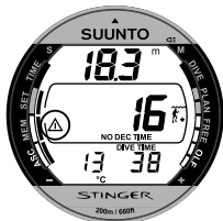
Fig. 3.7. Bookmark activation. An annotation, Bookmark, is placed in the profile memory during a dive by pressing the S button (Displayed with Diver Attention symbol.).
