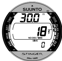
Fig. 3.9. Planning. The no-decompression time limit at 30.0 m [100 ft] is 18 minutes in P0/A0 mode.
