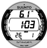
Fig. 3.29. Free dive. Present depth is 6.1 m, dive time 1.03 min and dive number is 1.
