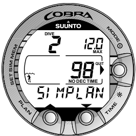
Fig. 4.21. Dive Planning Simulation.
