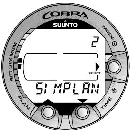
Fig. 4.19. Dive Planning Simulator mode. [2 SIMPLAN].
