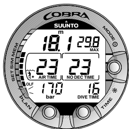
Fig. 3.26. The lowest bar graph blinks to indicate that the OLF value shown relates to OTU.
