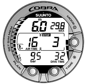
Fig. 3.11. A three minute Recommended Safety Stop.
