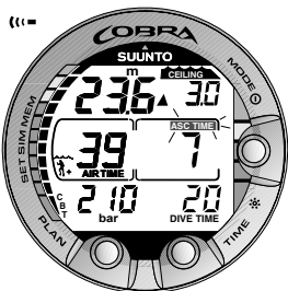
Fig. 3.16. Decompression dive, below floor. Upward pointing arrow, blinking ASC TIME label and an audible alarm tell you to ascend. Minimum total ascent time including safety stop is 7 minutes. Ceiling is at 3 m [10 ft].
