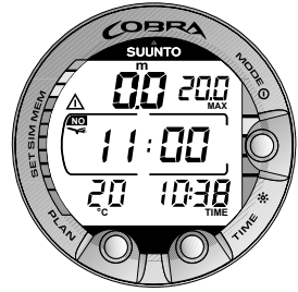
Fig. 3.30. Surface interval, no-flying time. Pressing TIME button twice will show no-flying time, indicated by an airplane symbol.
