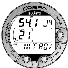
Fig. 3.21. Nitrox display. Maximum depth based on set O_2\% (21%) and PO_2 (1.4 bar) is 54.1 m [177 ft].
