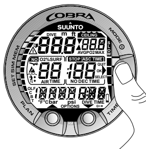
Fig. 3.1. Startup I. All segments shown.
