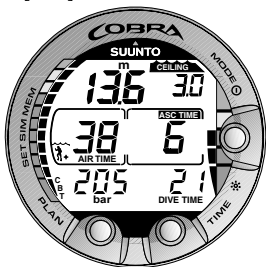
Fig. 3.17. Decompression dive, above floor. Upward pointing arrow has disappeared and ASC TIME label has stopped blinking, which means that you are in the decompression range.
