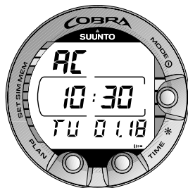
Fig. 2.4. Active water contacts are indicated by the text AC.
