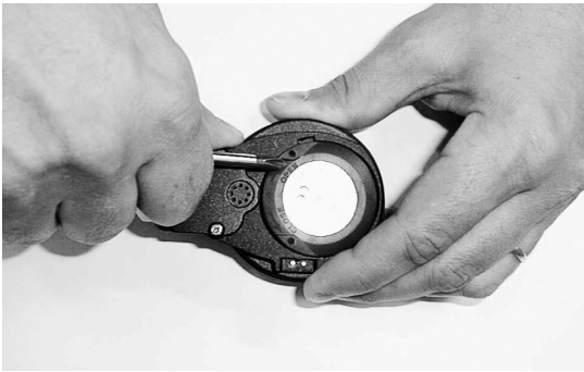
Fig. 5.3. Opening of securing ring.
