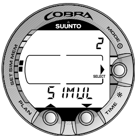
Fig. 4.3. Simulation option. [2 SIMUL].
