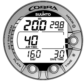
Fig. 3.27. Diving in Gauge mode.
