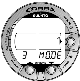
Fig. 4.1. Main menu based Mode options. [3 MODE].
