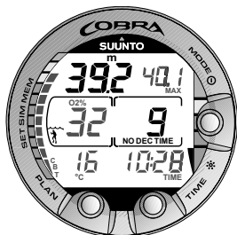
Fig. 3.25. Alternative display. Pressing TIME button displays current time, maximum depth, temperature, CBT and O 2 %, if Air Time is less than 30 minutes.
