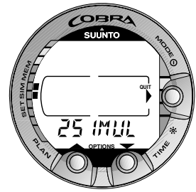
Fig. 4.16. Dive Simulation options. [2 SIMUL].
