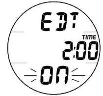
Fig. 30 - SET EDT ALARM
