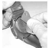
Fig. 70A - BATTERY COVER REMOVAL (using tool)
