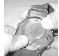
Fig. 74B - COVER INSTALLATION (without tool)
