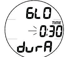
Fig. 37 - SET BACKLIGHT DURATION
