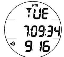
Fig. 4A - DEFAULT TIME (Main selected, no Dual)
