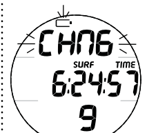
Fig. 64 - FREE SURFACE LOW BATT ALARM
