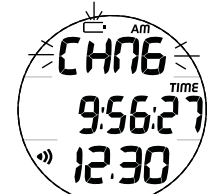
Fig. 60 - WATCH LOW BATTERY ALARM
