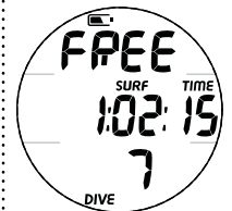
Fig. 63 - FREE SURFACE LOW BATT WARNING
