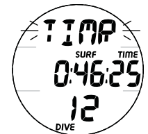
Fig. 61 - FREE SURFACE CDT ALARM
