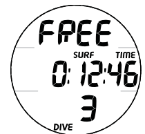
Fig. 21C - SURF MAIN (> 10 min after surfacing)
