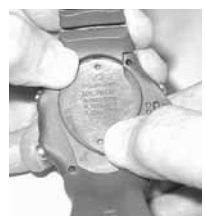
Fig. 70B - BATTERY COVER REMOVAL (without tool)
