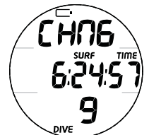
Fig. 3 - LOW BATTERY ALARM
