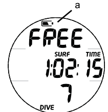
Fig. 2 - LOW BATTERY WARNING
