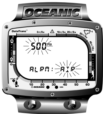
Fig. 18 - Air Alarm Setting
