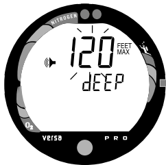
Fig. 21 - Set Max Depth Alarm
