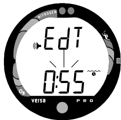
Fig. 22 - Set Elapsed Dive Time Alarm
