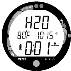
Fig. 16 - Surface Mode (rinse and dry the unit)
