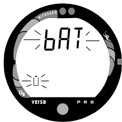
Fig. 9 -Low Battery Condition
