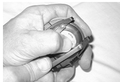
Fig. 90 -Ring Removal (alternate)
