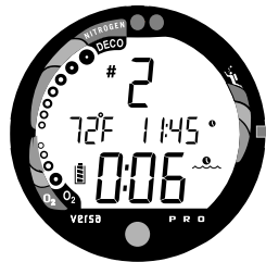
Fig. 60 - Immediate Violation Gauge Mode (after surfacing)
