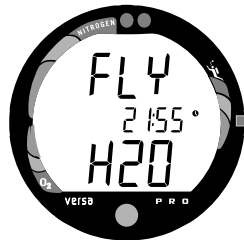
Fig. 75 - Fly Mode (Activation Contacts Wet)
