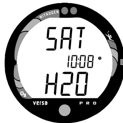
Fig. 76 - Desaturation Mode (activation contacts wet)
