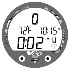
Fig. 9 -Low Battery Condition
