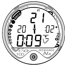
Fig. 37 - DECO STOP MAIN
