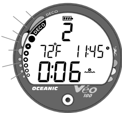
Fig. 34 - Violation Gauge Mode (on surface)
