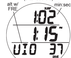
Fig. 128 - FREE VIOLATION (after 1 min on surface)
