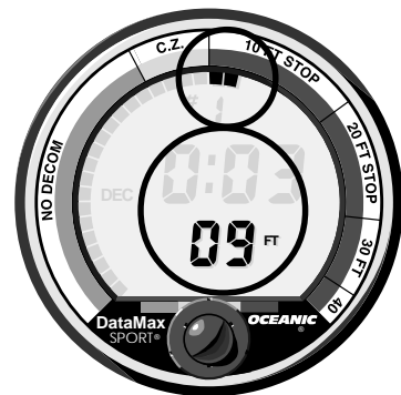
Fig. 23 – Depth less than required ceiling causes a Conditional Violation
