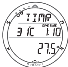
Fig. 138 - FREE DIVE MAIN (During CDT ALARM)
