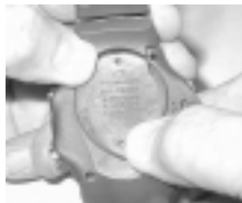
Fig. 145 - ALTERNATE HATCH REMOVAL
