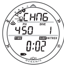
Fig. 4 - LOW BATTERY ALARM
