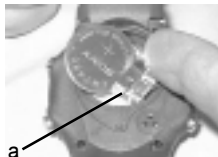
Fig. 146 - ATOM BATTERY REMOVAL
