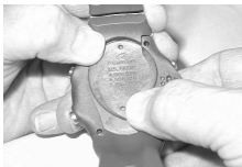
Fig. 118B - Alternate Battery Hatch Removal
