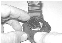
Fig. 121 - ATOM Battery Installation
