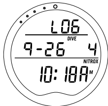
Fig. 115 - Log Preview (during Transition Period)
