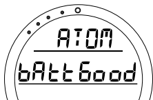
Fig. 5 - Battery Status (Good)
