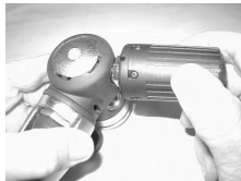
Fig. 127 -Threading Transmitter into Regulator
