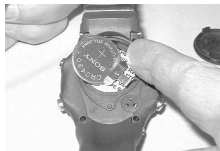
Fig. 119 - ATOM Battery Removal
