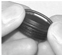
Fig. 124 - Transmitter O-ring Installation
