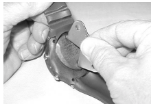
Fig. 118A - ATOM Battery Hatch Removal
