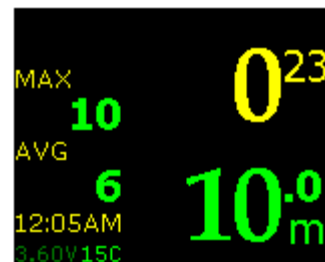
Battery Meter: Voltage
