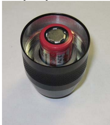
Insert the spacer with the battery into the battery compartment
