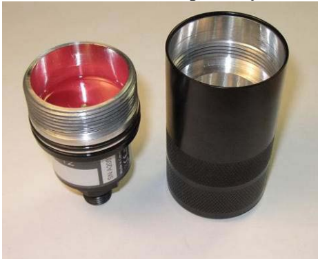
Replace the regular U-2 battery top with the extended U-2 battery top
