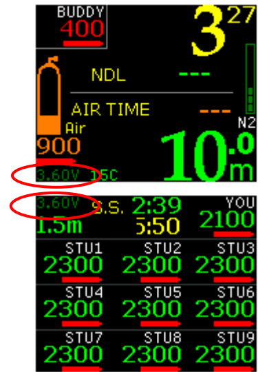
LYNX Battery Meter: Voltage
