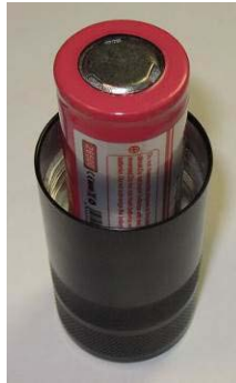
Load the IMR26500 into the battery top
