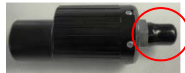
Transmitter with protective cap – ready to store!
