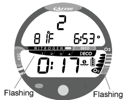
Fig. 60 - Immediate Violation Gauge Mode (after surfacing)
