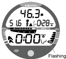
Fig. 63 - High O2 Warning
