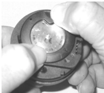
Fig. 58 -Engaging Retaining Ring
