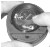
Fig. 56 -Inserting Retaining Bar
