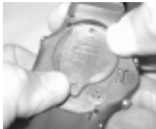
Fig. 151 - ALT BATTERY HATCH INSTALLATION
