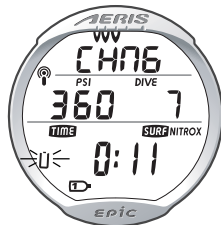
Fig. 4 - LOW BATTERY ALARM
