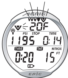
Fig. 99 - DELAYED VIOLATION #1 MAIN
