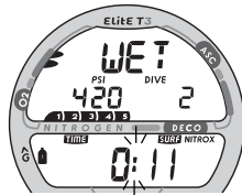
Fig. 16 - NORM SURF MAIN (post dive, unit wet)
