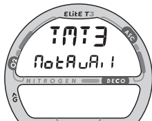
Fig. 6 - Transmitter 3 Status (Not Available)
