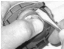
Fig. 130 - TIGHTENING Elite T3 HATCH RING
