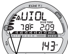
flashing Fig. 122 - FREE DIVE MAIN (During DECO)
