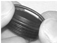
Fig. 131 - TRANSMITTER O-RING INSTALLATION
