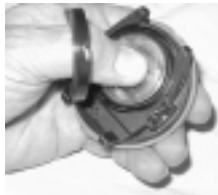
Fig. 129 - Elite T3 BATTERY INSTALLATION
