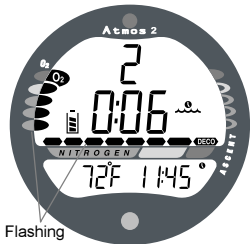
Fig. 57 - Immediate Violation Gauge Mode (after surfacing)
