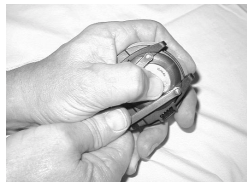
Fig. 45 - Hatch Ring Installation
