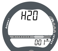
Fig. 8 - Surface Mode (rinse and dry the Atmos 1)
